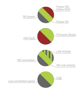
The LEDs indicate the following states of the motioncam:
