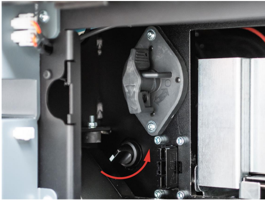
Figure 2.11. Turn the Manual brake release switch counter-clockwise to release the brakes.
