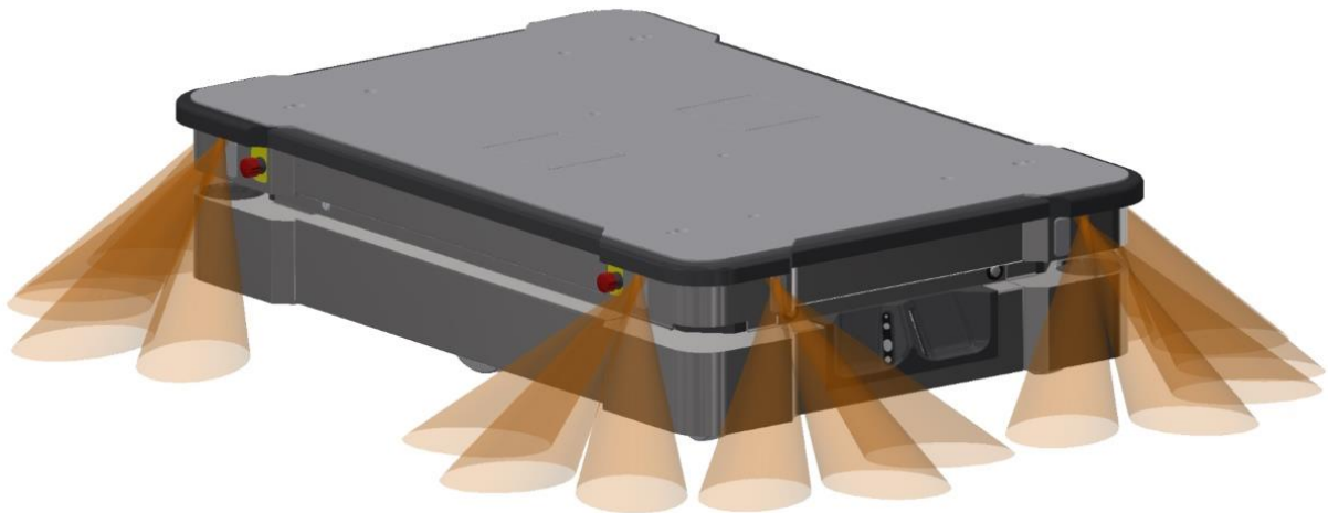
Figure 9.10. The proximity sensors in the corners of the robot detect objects below the safety laser scanners' plane of view.
