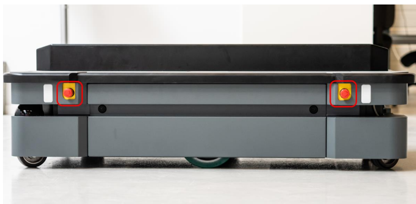
Figure 10.1. MiR500 has four Emergency stop buttons and the option to connect additional Emergency stop buttons through the electrical interface.
