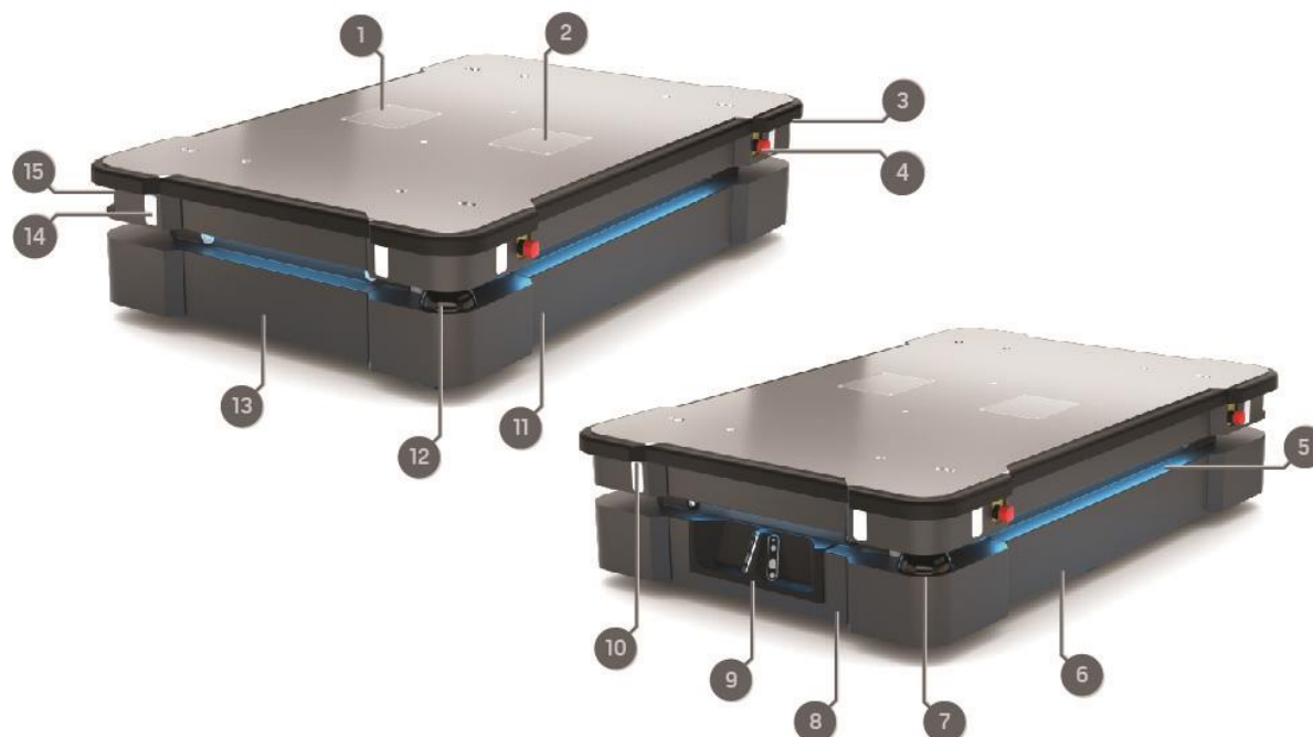
Figure 2.1. MiR500 external parts.
