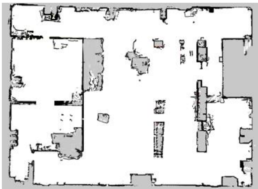
Figure 9.3. Example of a map that includes too much noise and dynamic obstacles.
