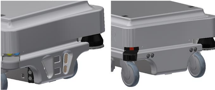
Figure 7.10. Two ultrasound sensors are placed at the front of the robot (left) and two at the rear of the robot (right).
