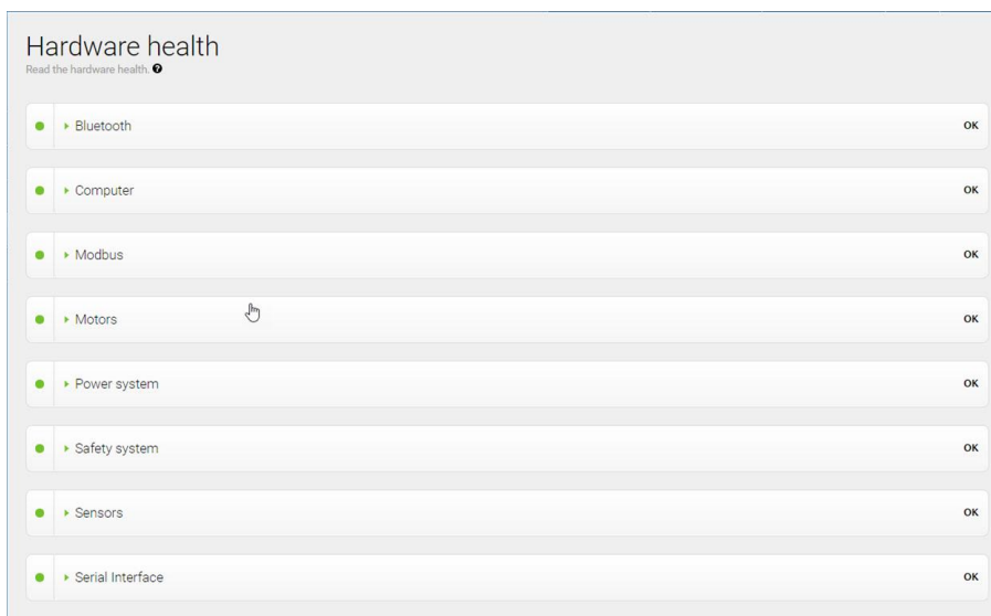
Figure 17.1. The interface in Hardware health displays which component is failing and often for what reason.
