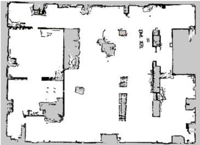
Figure 11.3. Example of a map that includes too much noise and dynamic obstacles.
