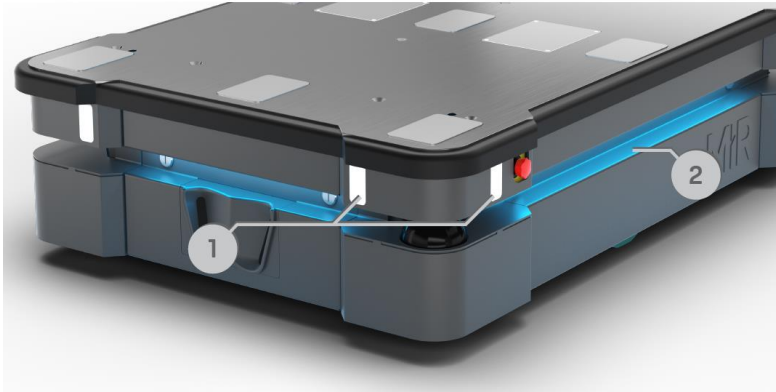
Figure 10.13. Indicator lights on MiR600.
