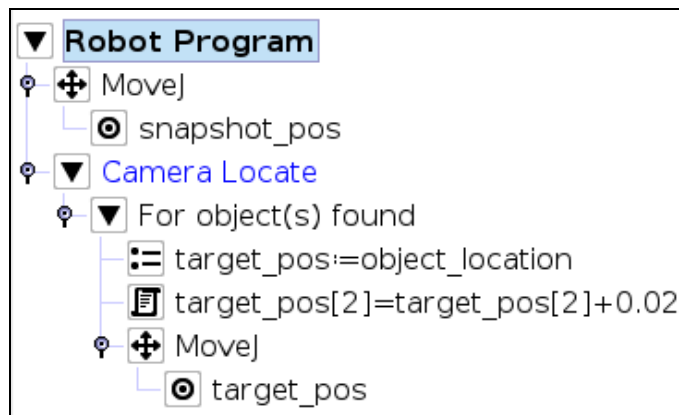
Fig. 8-12: Program example – Place the TCP 20 cm above the detected object, in case of an horizontal plane. e-Series robot program is illustrated.
