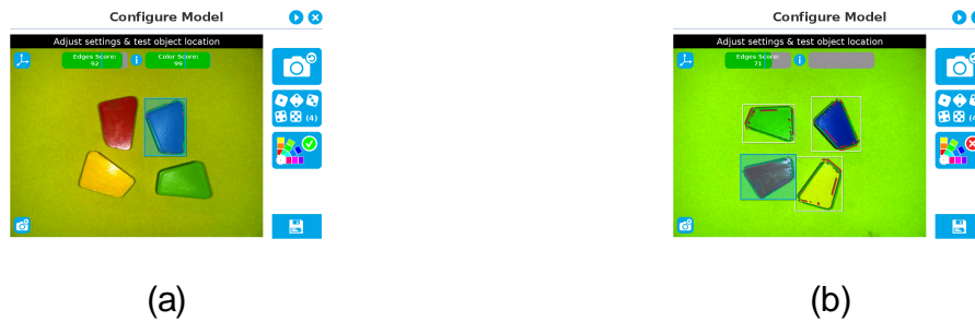
Fig. 7-36: Examples of Edges Score for (a) a blue part (b) a red part.
