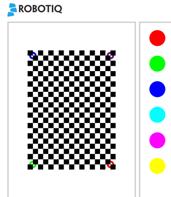
Fig. 6-4: This side of the calibration board is used for UR3 Universal Robots models. Color dots are not currently used by Robotiq software.
