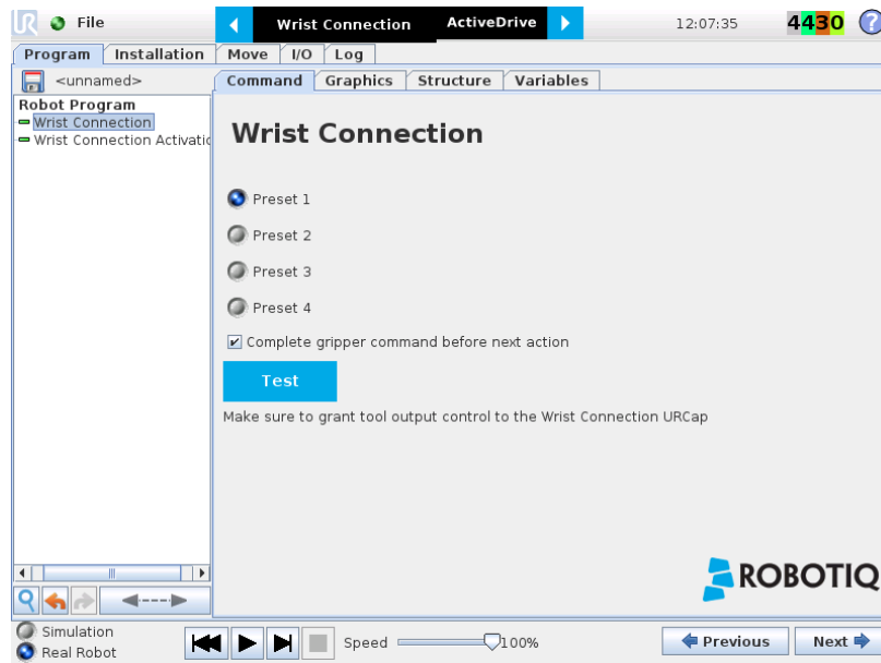
Fig. 4-5: Wrist Connection Node Interface.
