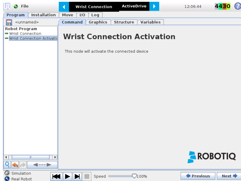
Fig. 4-4: Wrist Connection Activation Interface.
