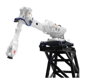
The IRB 6650S is the shelf robot form of the Power Robot family which offers a unique working envelope. It is capable of a full vertical and horizontal stroke motion, as well as an increased forward and downward reach. This combination offers new possibilities to robot functions in numerous application areas.
