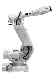
IRB 6640 Foundry Prime robot is designed for washing and cleaning applications. It is based on proven components from earlier generations, to ensure ease of maintenance and exchangeability as well as high up time.
