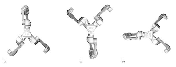
01 Working area ±135° with robot foot mounted on floor/ top of pillar.
