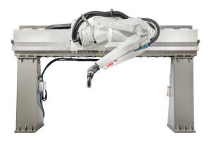
The Elevated Rail for the IRB 5500 reduces cycle times by as much as 10% on Stop & Go automotive paint lines.
