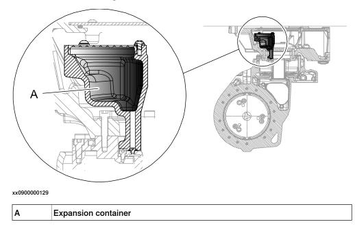
1.3.4 Expansion container for inverted mounting of the manipulator *Continued*
