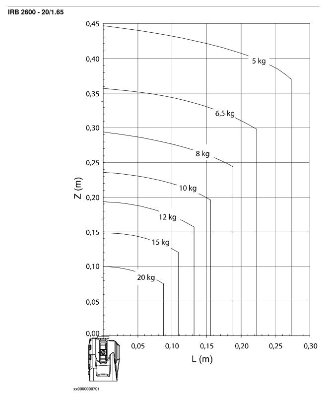
Extra load of 10 kg at the upper arm housing and 1 kg at wrist included in the load diagram.
