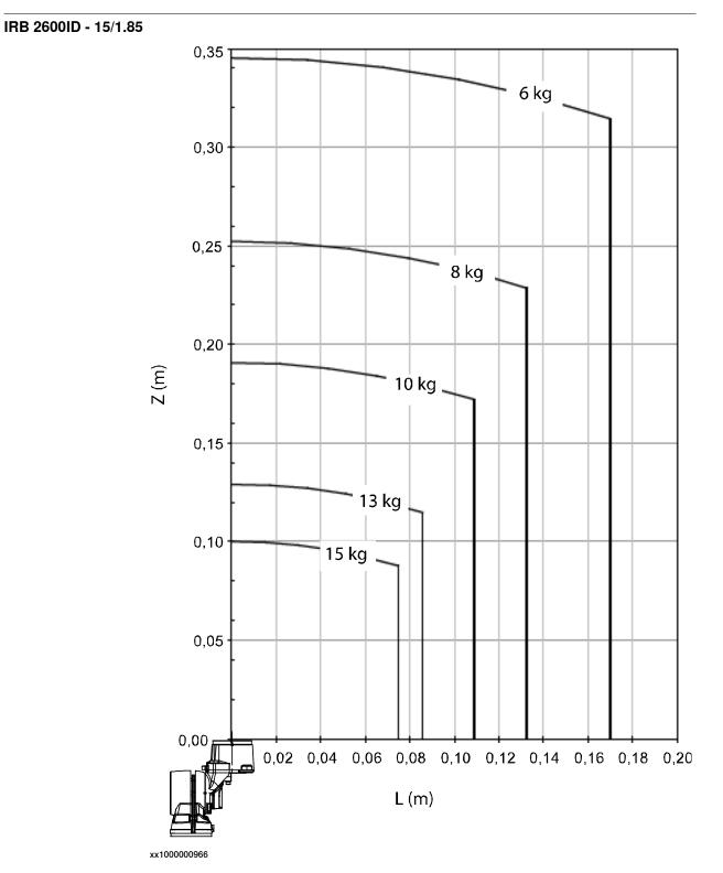
Extra load of 10 kg at upper arm and 1 kg at wrist included in the load diagram.
