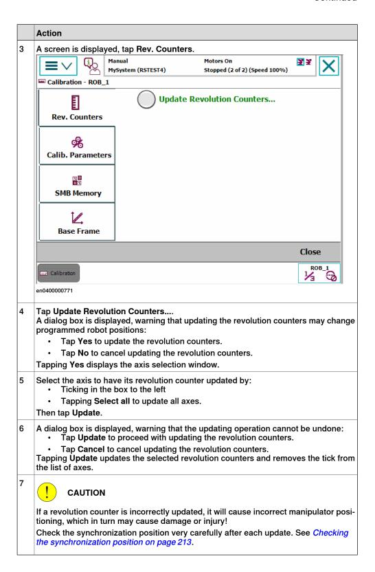
5.6 Calibrating with Calibration Pendulum method
