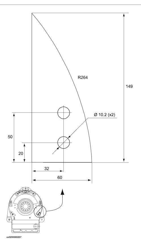
2.4.3 Mechanically restricting the working range of axis 2
