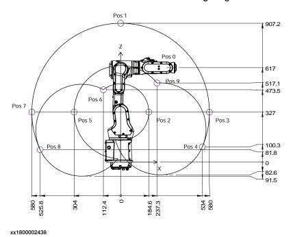
Positions at wrist center and angle of axes 2 and 3
