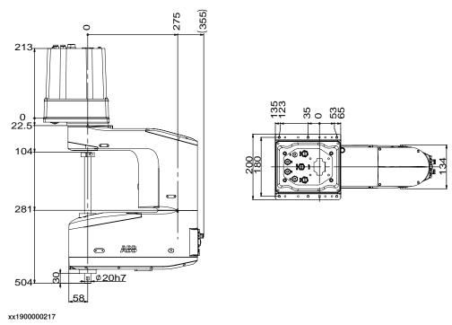
Robots with protection class IP54 (option 3350-540) or with protection type Clean Room (option 3351-1) The figure shows the dimension of the IRB 910INV-6/0.55 for Clean Room/IP54.
