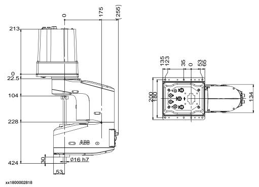
Robots with protection class IP54 (option 3350-540) or with protection type Clean Room (option 3351-1)
