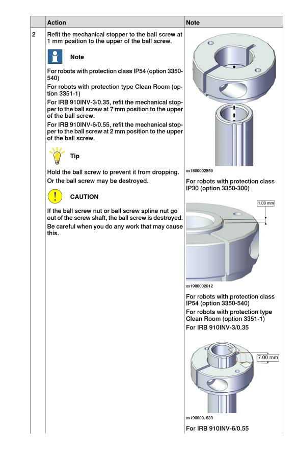
5.6.1 Replacing the mechanical stopper *Continued*
