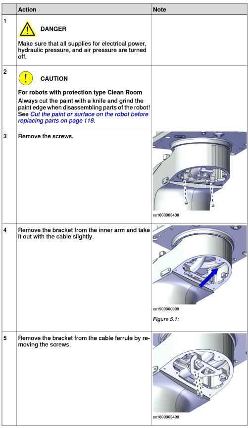
Action Note 1 DANGER Make sure that all supplies for electrical power, hydraulic pressure, and air pressure are turned off. 2 CAUTION For robots with protection type Clean Room Always cut the paint with a knife and grind the paint edge when disassembling parts of the robot! See Cut the paint or surface on the robot before replacing parts on page 118. 3 Remove the screws. 4 Remove the cable ferrule on the cable and take it out. xx1800003410
