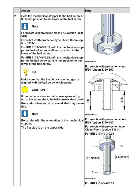
5.6.4 Replacing the pulley on the ball screw lower position *Continued*
