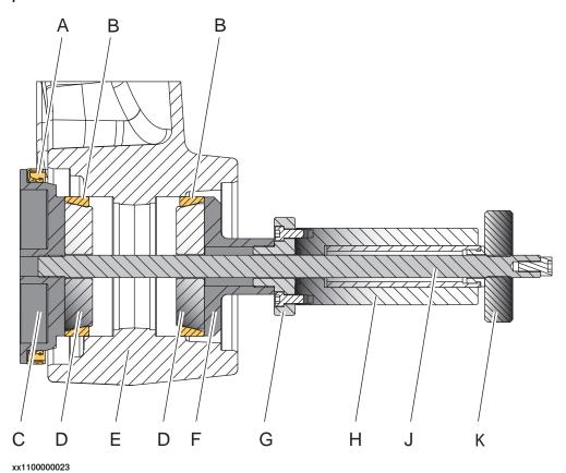
Α Radial sealing with dust lip D=120 mm/140 mm, T=13 mm В Bearing, outer race (2 pcs) С Mandrel, bearing and seal D Guide (2 pcs) Ε Link F Pressring, bearing G Distance Н Hydraulic cylinder J Connecting rod Κ Stop nut M16 D=80 mm, T=20 mm
