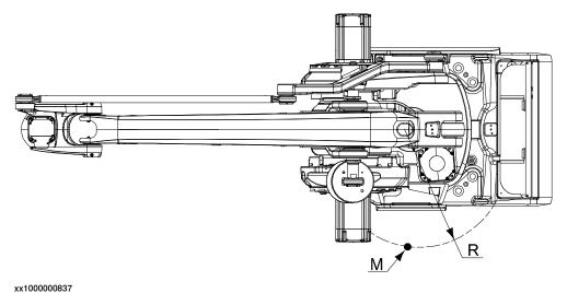
The following figure shows the radius for extra load on frame.
