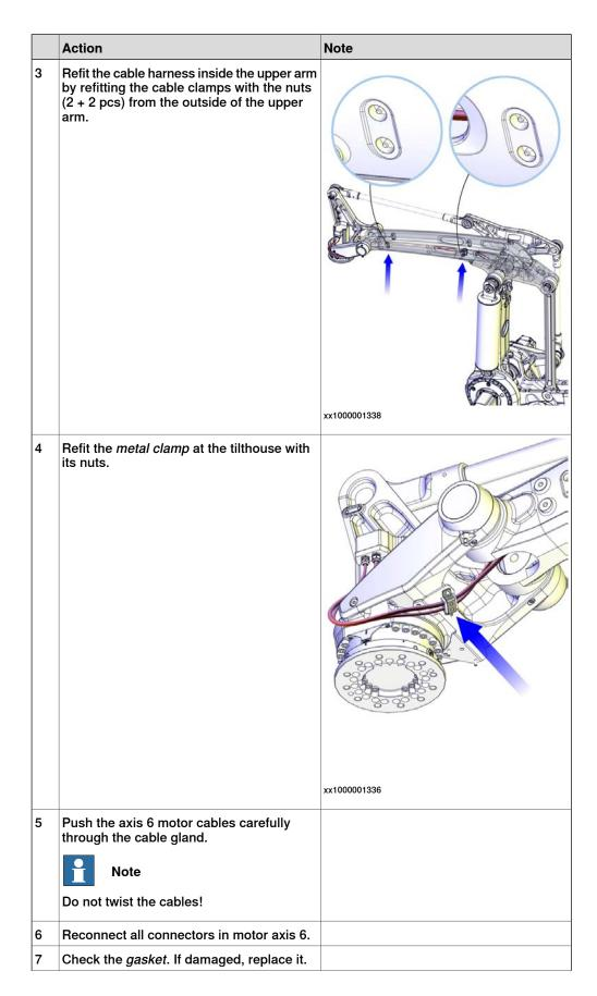
4.3.2 Replacing the cable harness, upper end (incl. axis 6) *Continued*
