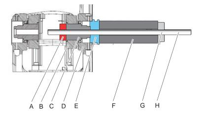
(shown as A) in the figure must be used when fitting the shaft. If not the shaft will not be pressed in completely.
