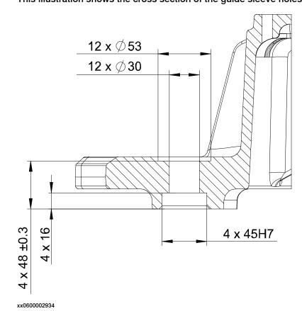
Cross section, guide sleeve hole This illustration shows the cross section of the guide sleeve holes.
