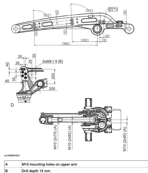
**Note**! The weight of the extra equipment on the upper arm must be deducted from the maximal handling capacity.
