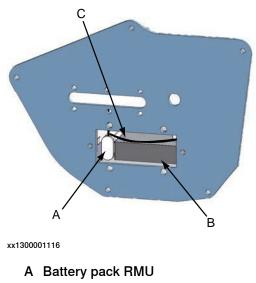
Battery pack with a 3-pole battery contact (RMU)
