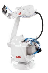
The IRB 52 is a compact painting robot designed specifically for painting small and medium sized parts in a wide range of industries. It provides you with an affordable, professional and high-quality painting solution.
